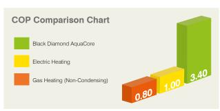
Heat pumps use electrical energy and take low grade heat energy from the outdoor air, to heat refrigerant which in turn heats water for domestic use. The efficiency of a heat pump is known as the Coefficient of Performance or COP. This is a ratio of the heat delivered to power consumed. For every 1kW of electrical input energy, the heat pump absorbs renewable heat energy from the outdoor air to provide the home with an average of at least 3.4kW\*3 of heat output.
